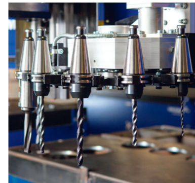
The drill with multiple tool changer produces accurate holes and even taps threads.
