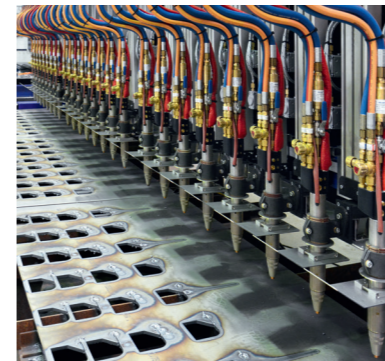
The machine can be equipped with a maximum of 24 oxyfuel torches.
