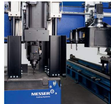
Drilling, boring, counter-sinking and thread tapping as additional processing possibilities
