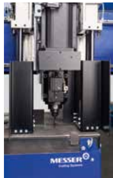
Drilling, boring, counter-sinking, tapping as additional processes
