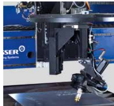
The plasma bevel cutting unit Skew Rotator Infinity facilitates the immediate cutting of bevels on parts
