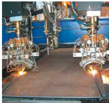
The triple torch bevel unit DAFL is the ideal tool for cutting wind tower plates
